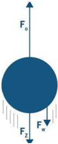
Figure 46 The forces that are exerted on a rising emulsion droplet.
