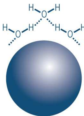
Figure 30B Water molecules around an oil droplet
