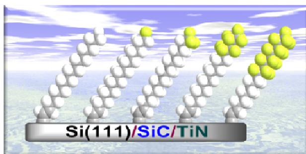
**Figure:1** Schematic representation of fluoro-hydro monolayers on Si(111), SiC and TiN.
