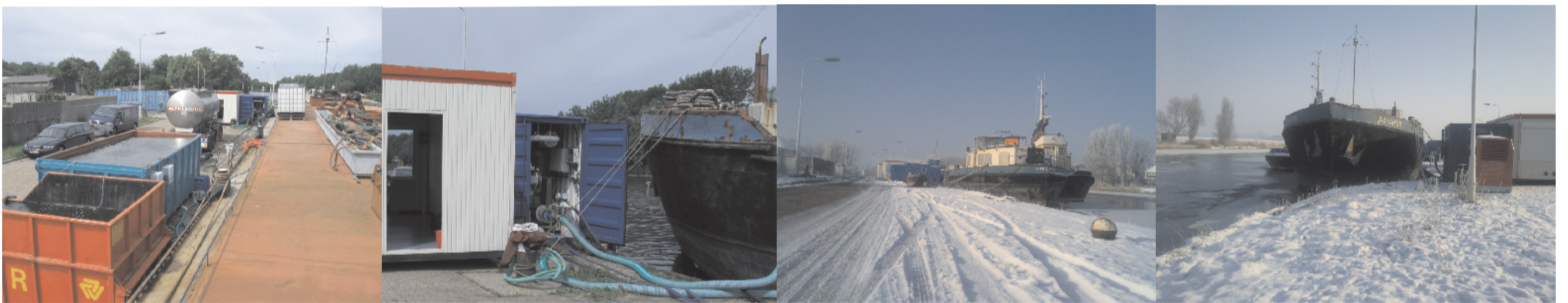
Hamworthy land-based test site in the Netherlands, with additional phytoplankton cultures and BWMS next to the laboratory container. The barge Aquarius has over 400 m 3 storage capacity. Additional cultures facilitate year round land-based testing, provided icing does not make working at the test site too dangerous.
