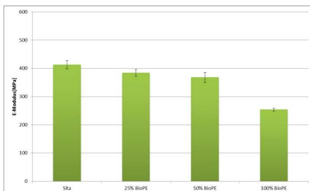
Figure 2 E modulus of recyclates (references and samples containing bio-PE)
