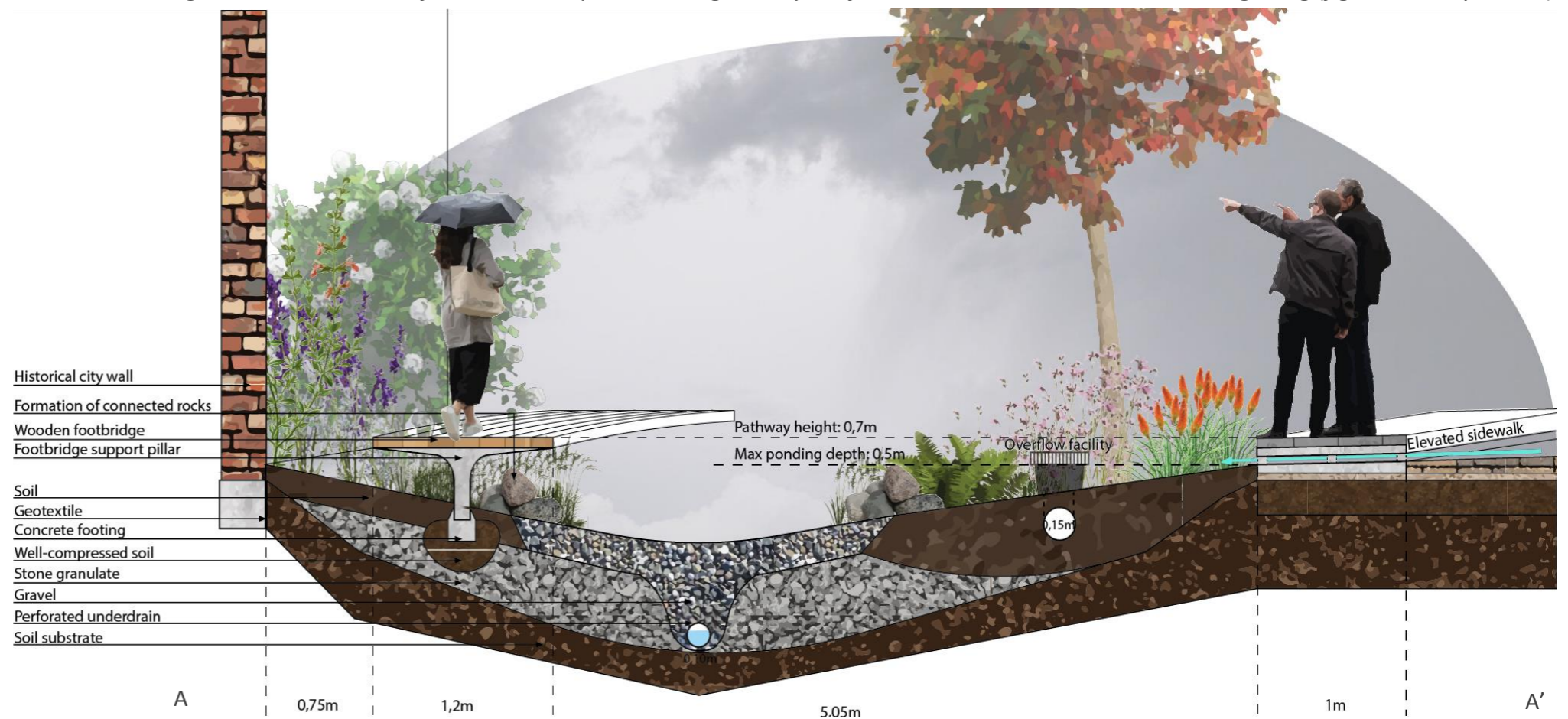
Figure 58: Cross-section of rain garden De Vestingtoren in vulnerable area The Bokkingshang (figure made by author)
