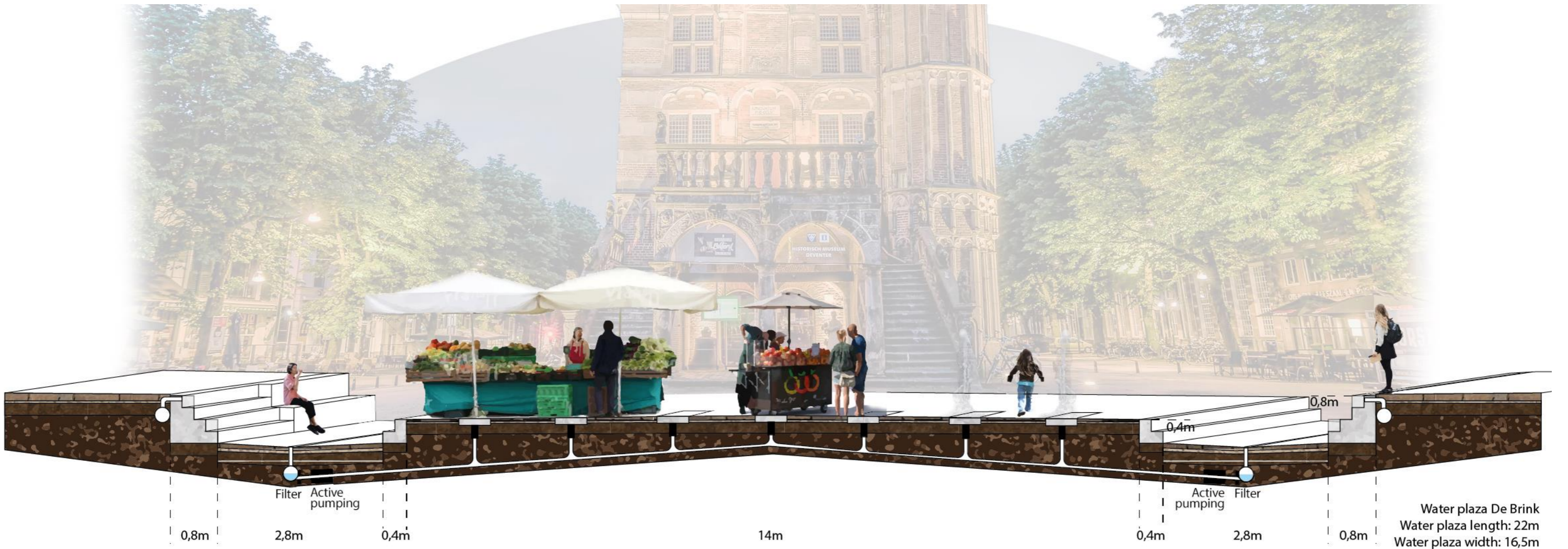
Figure 53: Cross-section of the water plaza in vulnerable area The Bokkingshang (figure made by author)
