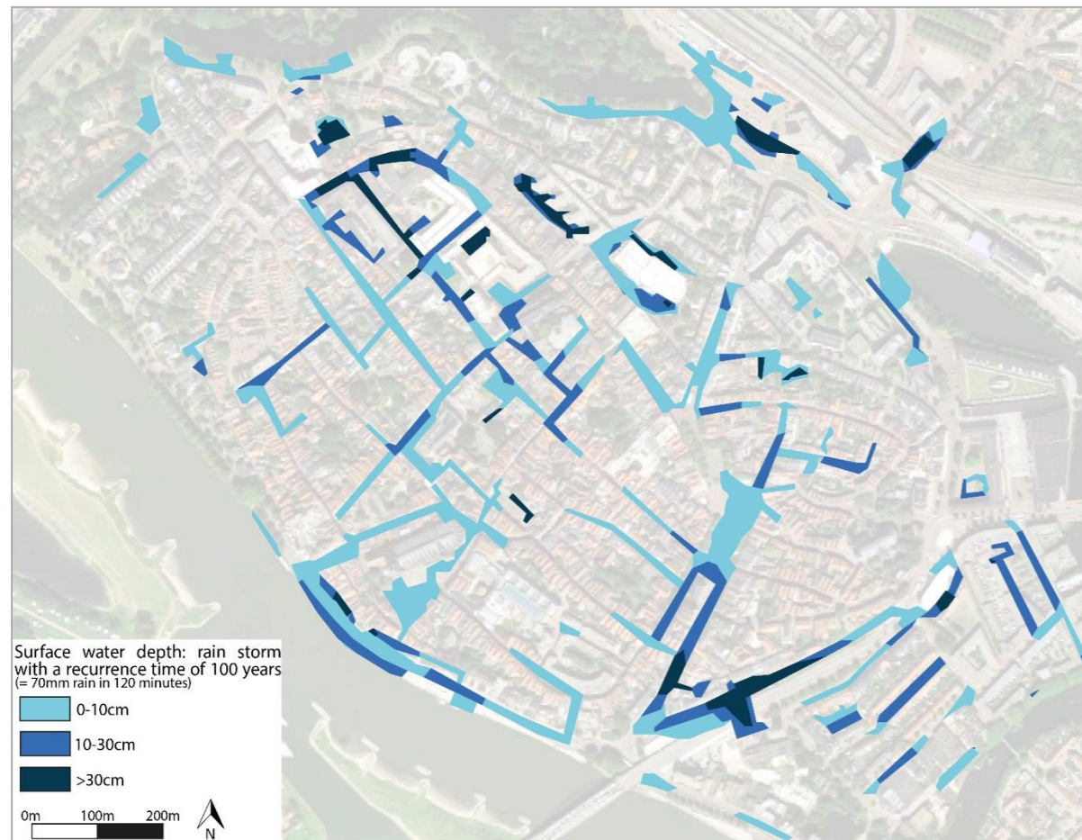
Figure 30b: Surface water depth after a rainstorm of 1 in 100 years (figure made by author)
