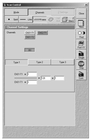
Fig. 5-60 Channel Settings panel of a Ratio Channel
