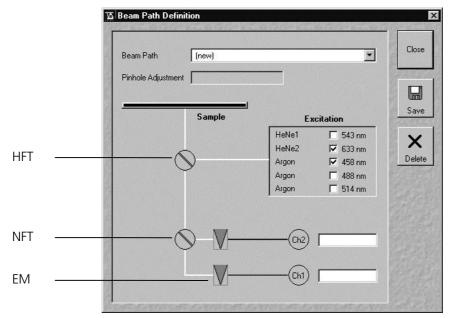
Fig. 5-207 Beam Path Definition window
