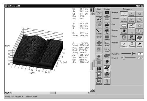
Fig. 5-336 Image Display window, Topography display: 3D - Volume
