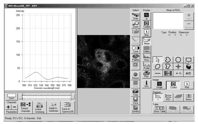
Fig. 5-348 Image Display window of a Lambda Stack, Display - Mean activated
