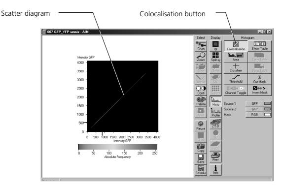
Fig. 5-303 Image Display window, Colocalization display
