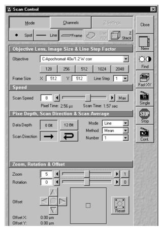
Fig. 5-394 Settings at the LSM control
