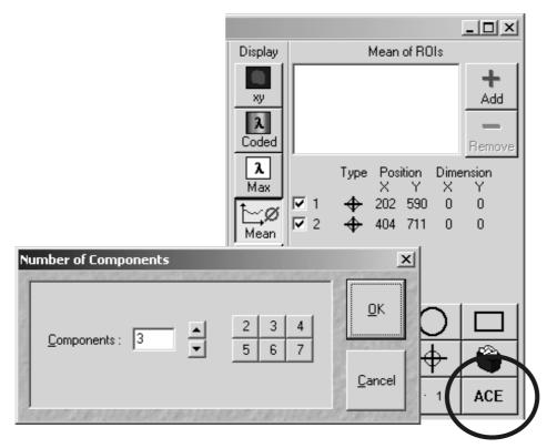
Fig. 5-349 Automatic Component Extraction function
