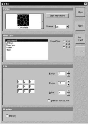
Fig. 5-124 Filter window (User-defined filter)
