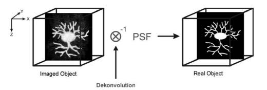
The effect of 3D deconvolution can be demonstrated impressively on objects with a known form. As a rule fluorescent beads are used for this purpose. The following figure shows the 3D deconvolution of an image stack with a fluorescent bead with a diameter of 1  $\mu$ m.
