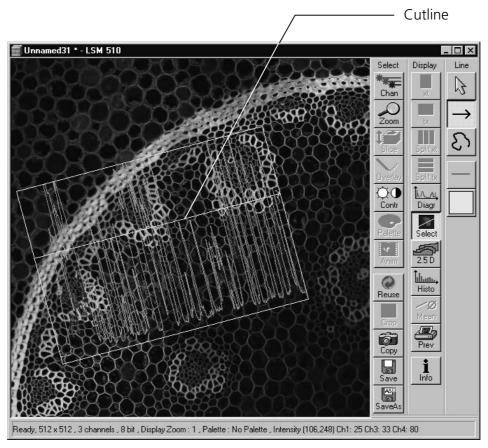
Fig. 5-68 Image Display window with cutline displayed
