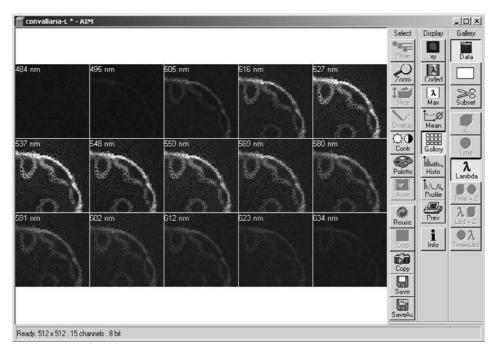
Image Display window with a Lambda Stack Fig. 5-64
