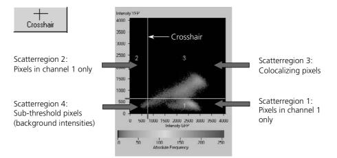
Fig. 5-305 Scattergram and thresholding with crosshair
