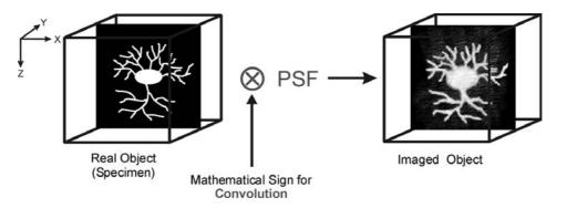
The **Point Spread Function** describes how the light of a point object is distorted by the optical system. This "convolution" makes the image appear grainy and structures in the image seem blurred. This effect is most prominent in the axial (Z-)direction as each lens is optimized for the two-dimensional image of the object.
