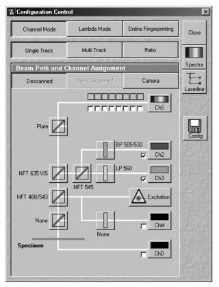
Fig. 5-362 Configuration Control window
