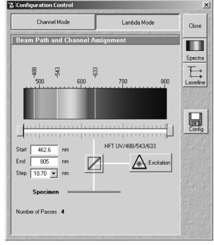
Fig. 5-50 Configuration Control window; Lambda Mode activated
