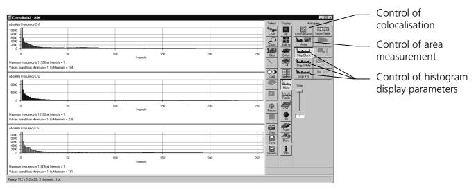
Fig. 5-298 Image Display window, Histogram display
