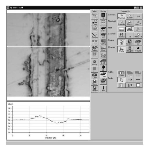
Fig. 5-333 Image Display window, Topography display: 2D - Profile
