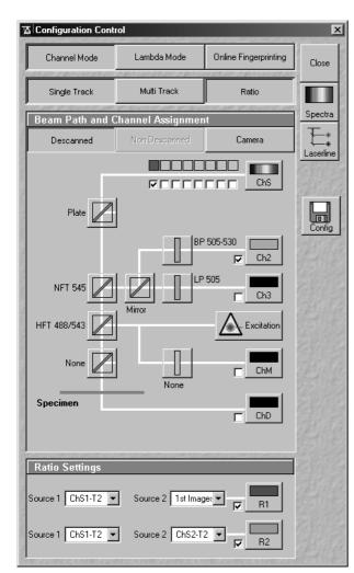
Fig. 5-49 **Configuration Control window;** Ratio activated
