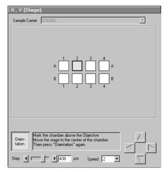
Fig. 5-167 X, Y (Stage) panel (Sample drives unlocked)
