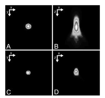
Fig. 5-140 Image of a fluorescent bead with a diameter of 1µm before deconvolution (A,B) and after deconvolution (C,D)
