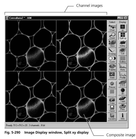
This function is useful to optimize the individual channels in a multi channel image acquisition together with the **Range Indicator** palette .
