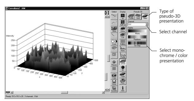
Fig. 5-310 Image Display window, 2.5 D display
