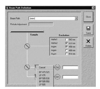
• Click on the **Emission Filter** symbol(s) I to get the list box allowing you to select the emission filters you need.
