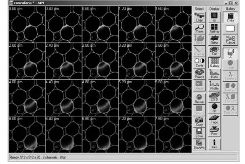
Fig. 5-73 Image Display window of a Z Stack
