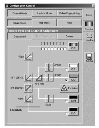
Fig. 5-350 Configuration Control window
