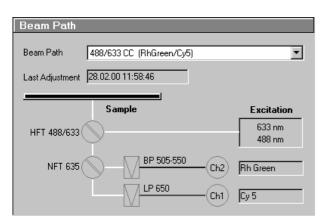
Fig. 5-200 Beam Path panel
