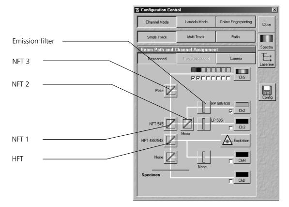
Fig. 5-41 Configuration Control window
