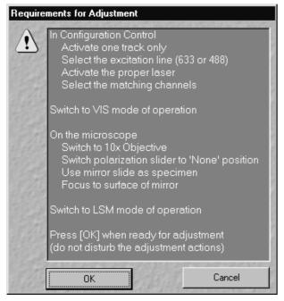
Fig. 5-264 Requirements for Adjustment window
