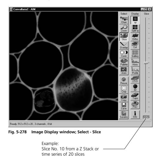
• Select the slices using the slider on the right.
