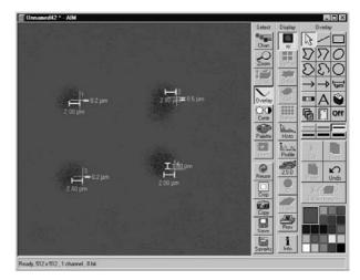
Fig. 5-399 LSM image after bleaching with overlaid distance markers
