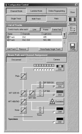
Fig. 5-46 Configuration Control window, Multi Track activated
