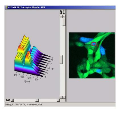
**Mono** button: Change between color and monochrome display of the intensity time diagrams over Lambda.
