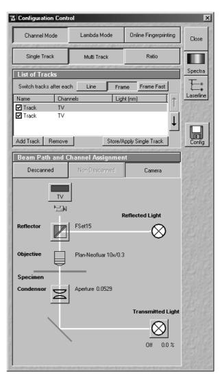
Fig. 5-52 Configuration Control window; camera detecting activated
