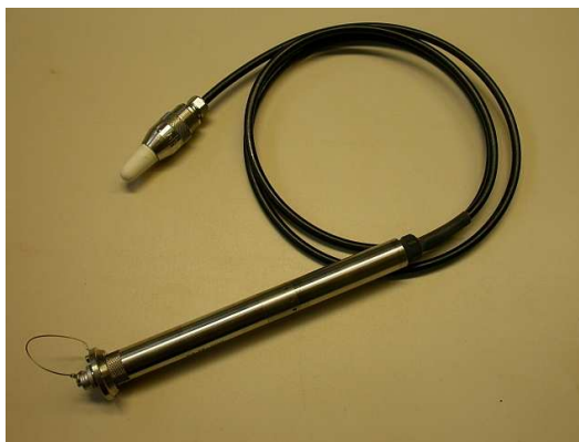
Fig. 1: picture of a polymer tensiometer including cable and data logger/power supply unit
