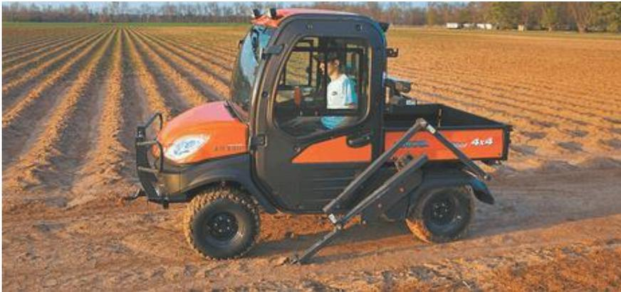
Rapidprobe Rtv equipped with Gps and autosteer
